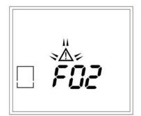
Fault of the decorative fire. The display shows an F, followed by a 2-digit fault code. The symbol  $\Lambda$  flashes.
