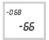
The RSSI (Receiver Signal Strength Indicator) values are shown. At the top left the RSSI of the remote control and at the bottom right the RSSI of the DFGT.
