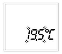
The current temperature set point flashes. Set the required set point by pressing key △ or ✓. Dependent on the key pressed, the symbol ∧ or ✓ is shortly shown on the display. The temperature can be set between 5,0 and 35,0 °C.
