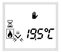
This display is shown. The symbol  $\checkmark$  flashes to indicate the decorative fire is being switched off. After the decorative fire has been switched off, the default display is shown again.
