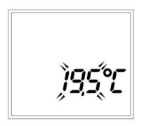
The current temperature set point flashes. Set the temporarily required temperature set point by pressing key ☐ or ☑. Dependent on the key pressed, the symbol or ☑ is shortly shown on the display.
