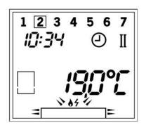
This display (example) is shown. Symbol flashes to indicate the decorative fire has to be ignited manually by pressing keys and simultaneously.
