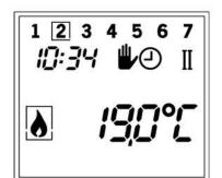
This display (example) is shown. The symbol windicates that the temperature set point has been adjusted manually.
